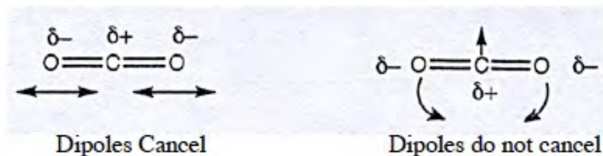
Fig. 6-7 Lewis structure of CO 2 , with opposite dipoles canceling one another when the molecule engaged in a symmetrical vibration, and creating a net overall dipole when the molecule is bent during a “wagging” vibration.
