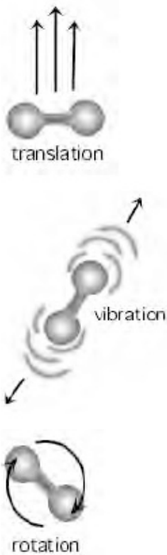
Fig. 6-5 Three different modes of molecular motion: translation, rotation and vibration. All three can occur at the same time.
